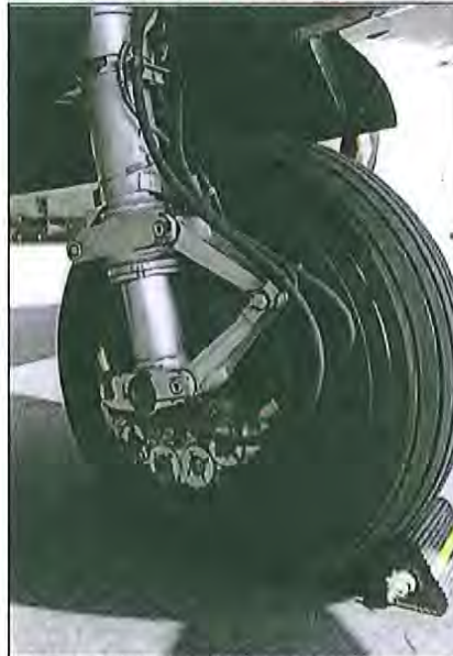
Each main landing gear has dual-redundant, three-piston disc brake callipers. An analog anti-skid system improves stopping performance on contaminated runways.
