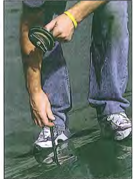
Each R-2800 engine consumes about one gallon of oil per hour. Accordingly, pilots plan on adding 24 quarts of oil to each left- and right-side 35-gallon wet-wing tank after a six-hour flight. Considerable oil seeps out of the engines after shutdown, so large drip pans are needed to prevent oil spills in the hangar. Operators buy oil in 55-gallon barrels for oil changes.
