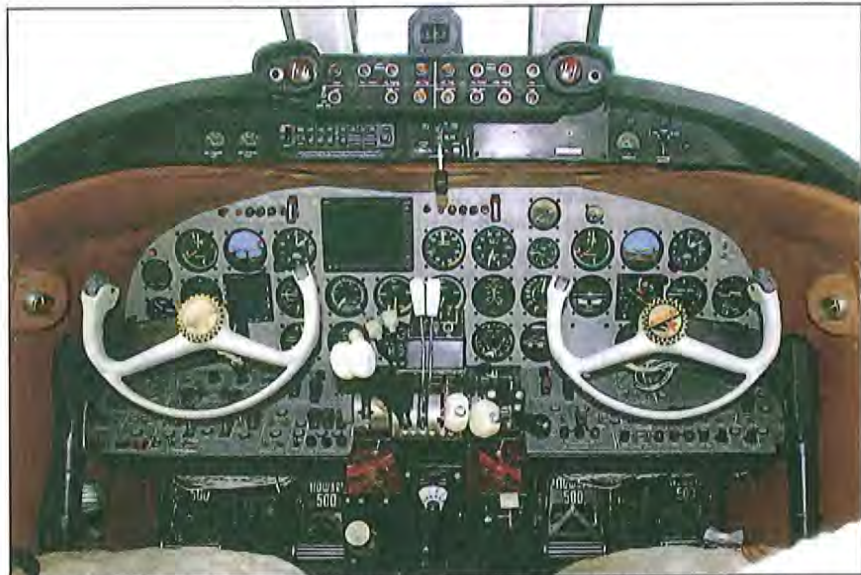
Look closely at the power quadrant and imagine the pilot workload. There are throttle, prop and mixture levers, plus controls for high and low blower, auxiliary hydraulics, flaps, fuel tanks and carb inlet heat, among others. The instrument panel has MAP, rpm, fluid quantity, oil pressure/temperature, carburetor inlet temperature, hydraulic pressure, CHT, fuel flow and BMEP gauges.
