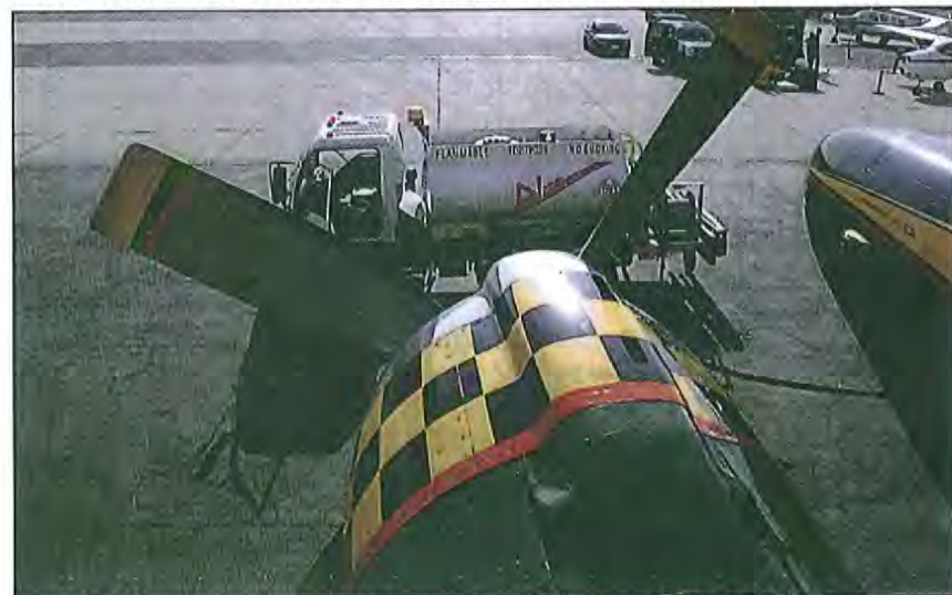
Huge engine nacelles, housing PW R-2800 engines, and 11-foot-diameter, four-blade props told everyone on the ramp in 1963 that the Howard 500 was the undisputed top dog among purpose-built, piston-engine business aircraft.
